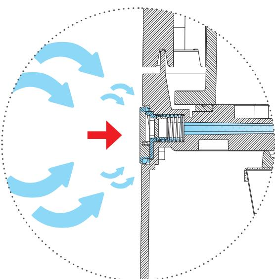
The valve opens automatically and facilitates the air flow to the motor.
