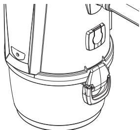
To use the service inlet, just insert the vacuum hose, without a micro-line connection.
